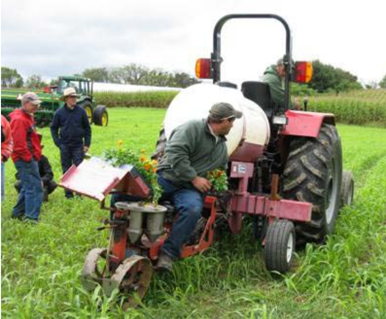
Whitney Scott (tractor driver), Delaware Valley College Horticulturalist and Alan Ard (sitting) of Ard's Farm Market west of Lewisburg, PA, demonstrate a no-till vegetable transplanter in a stand of sorghum-sudangrass during the field event. The transplanter is available for interested farmers for crops such as pumpkins, melons, etc.
