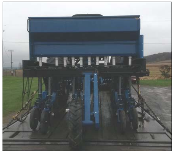
Farmers and researchers have been experimenting planting a cover crop between crop rows (such as field corn or sweet corn) while the crop is approximately "knee high." One piece of equipment that was tried in Snyder County was an interseeder (above), a no-till drill designed to plant between row crops spaced 30 inches apart. Farmers walk through an unharvested corn field where the interseeder was used during a Conservation District field day event (left). Notice the established cover crop between the corn rows (left and below).
