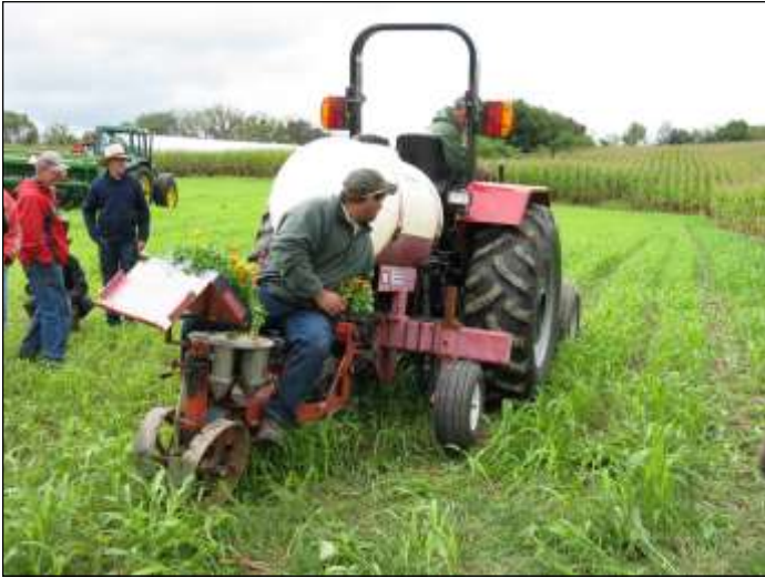
A team of four horses pull a no-till row planter (top left) and a no-till drill (top right) on harvested wheat fields during a Conservation District sponsored field day event. At center left, two farmers get ready to demonstrate how a no-till transplanter works during a Conservation District sponsored field day event. The no-till transplanter can plant seedlings such as pumpkin, tomatoes and squash.
